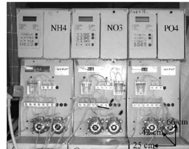
Fig. 1. MicroMac Fast MP3; module ammonia, nitrate and orthophosphate.
