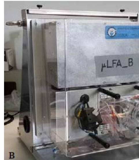
Fig. 4. The μLFA hydraulic circuit for fluorimetric phosphate analysis.
